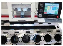
buttons and interactive menus required for a particular machine operation are displayed. Machine operations can easily be done manually or automatically, with the ability to store programs in memory. Digital readout allows the operator to accurately monitor position at all times. Control operates in metric and inch systems.
