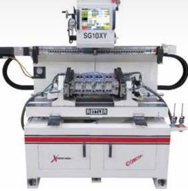
valve seat cutting such as valve seat housing counterboring and valve guide reaming, the spindle is required to be locked vertically. The ACTIV spindle has a pneumatic locking system that locks the spindle sphere rigidly vertically for other types of machining requirements.
