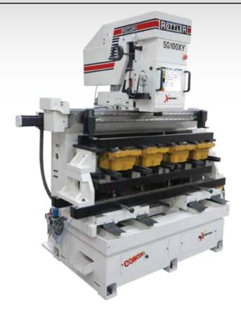
guide-to-guide automation for ease, accuracy and precision on even the largest heads. Rottler has developed fixtures that allow easy loading of four single heads and then, with one button operation, all heads are clamped at once. The fixture is designed to
