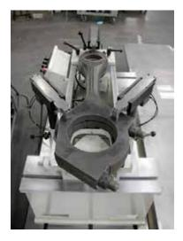
Special heavy duty fixtures available for boring very large, heavy connecting rods found in natural gas compressors and workboat marine engines are available.
